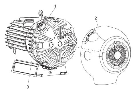
Fig. 21: Removing fan cover
