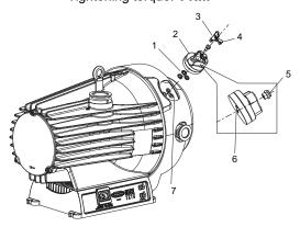
Fig. 27: Assembling gas ballast valve
