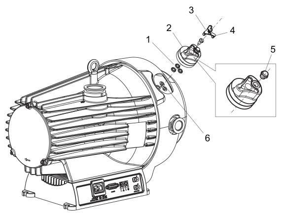
Fig. 24: Disassembling gas ballast valve
