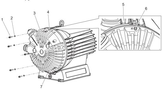
Fig. 28: Removing the spiral housing
