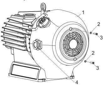
Fig. 19: Unscrewing and removing cylinder screws
