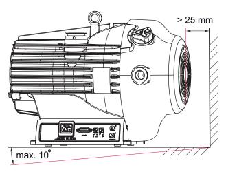
Fig. 5: Minimum distances and permissible inclination
