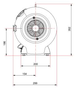
Fig. 34: Dimensions HiScroll 46 Dimensions in mm
