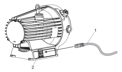
Fig. 9: Connecting to mains power supply
