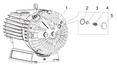
Fig. 22: Disassembling valves
