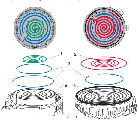
Fig. 29: Replacing tip seals on scroll pump
