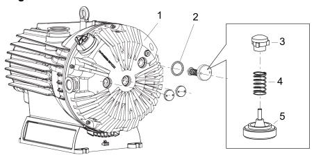
Fig. 23: Assembling valves
