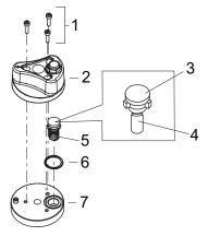
Fig. 26: Assembling gas ballast valve
