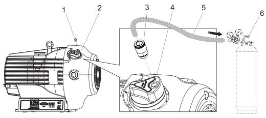
Fig. 8: Connecting gas ballast external supply
