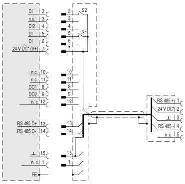
Connection diagram of 15-pin "remote" connection Fig. 11:
