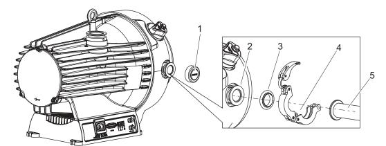
Fig. 7: Example of exhaust connection
