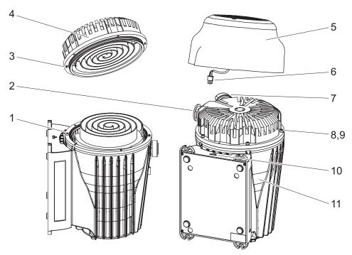
Fig. 31: Assembling the housing parts
